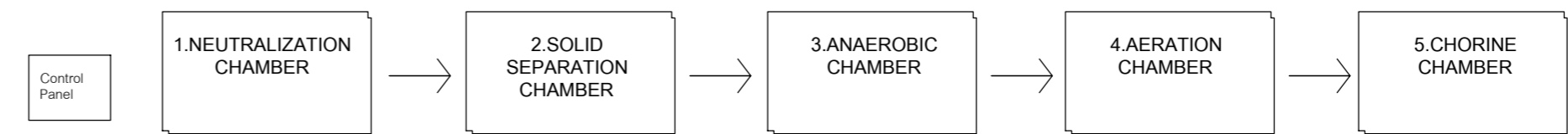
FLOW DIAGRAM OF CHEMICAL WASTEWATER TREATMENT PLANT
